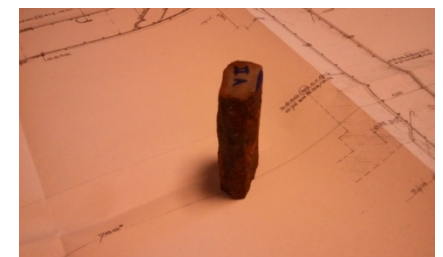
Steel bar with reduced cross section
