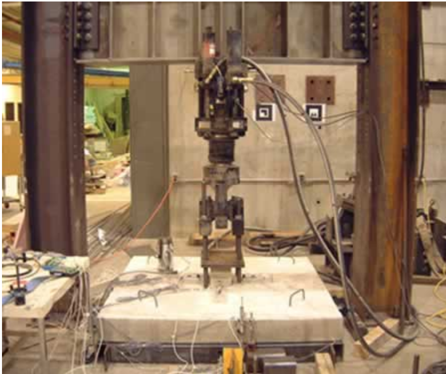
Traditional punching shear test on free slab specimen
