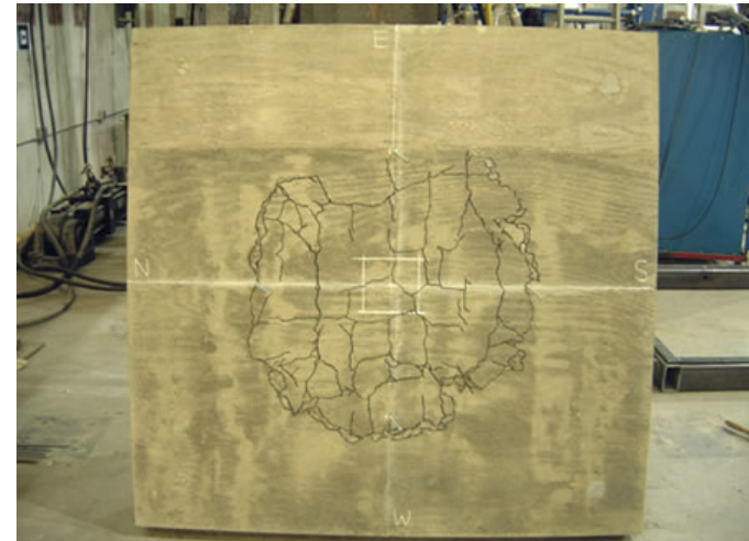
Traditional punching shear test on free slab specimen
